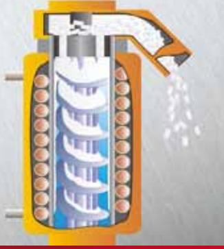
An evaporator screw rotates in an evaporation drum, which is filled with water and refrigerated from outside. The water freezes on the inner drum surface to small ice particles, which are scraped off by the rotating evaporator screw and conveyed upwards. The ice passes through an extrusion die and gets like that its characteristic nugget shape.
